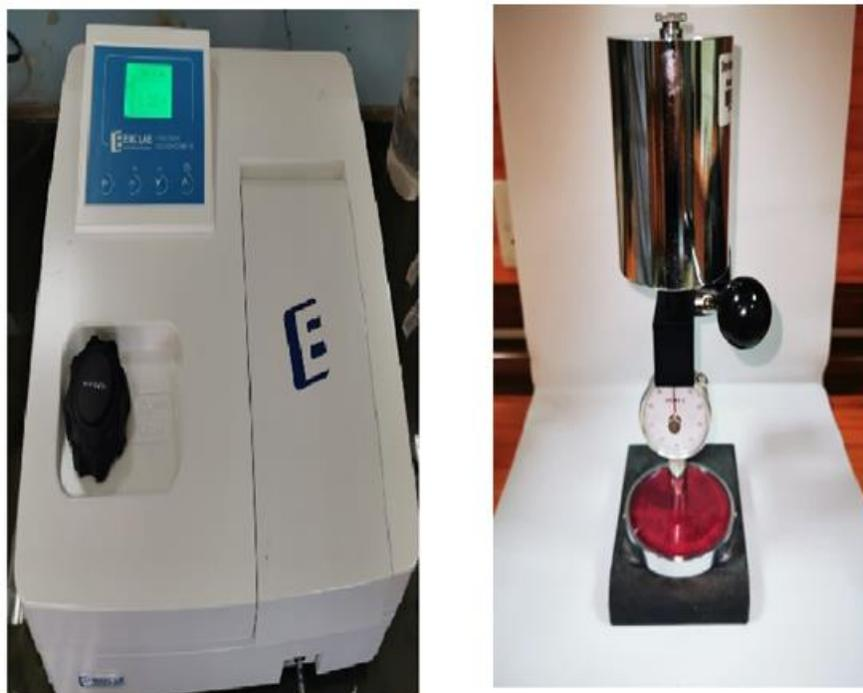
**Figure (1):** A-Spectrophotometer B-Shore A hardness measuring device
